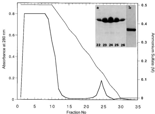
FIG. 4. Hydrophobic-interaction (phenyl-Sepharose) column chromatography profile of the Chi40s overproduced in BL21 *trx*(DE3) cells harboring the pECHChi40-9 construct and secreted in the growth medium. The bacterial supernatant was adjusted to 0.5 M ammonium sulfate and buffer B. Chi40s was eluted between 150 and 100 mM ammonium sulfate as the only symmetrical peak. Inset: (a) 0.1% SDS–15% PAGE and (b) native PAGE of the Chi40s peak fractions (for details see Materials and Methods).
