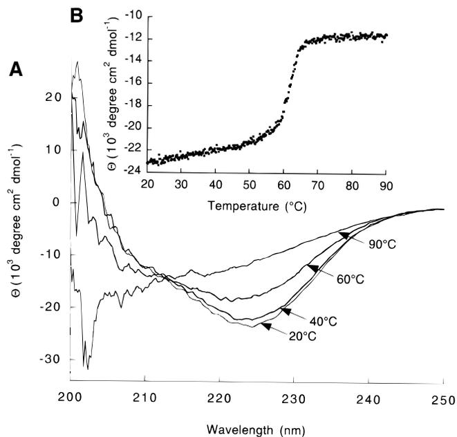
FIG. 5. (a) CD spectra of Chi40s at various temperatures as indicated. (b) Thermal melting curve of Chi40s as determined by CD spectroscopy at pH 7.0.
