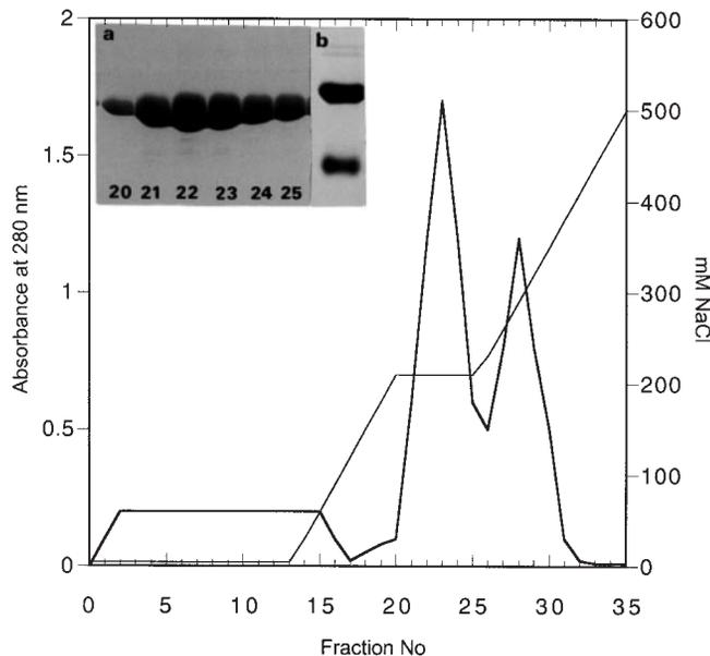
FIG. 3. Ion-exchange column chromatography profile of the Chi40c peak fractions from the Ni<sup>2+</sup> column on a Q-High Performance column at pH 8.0 in buffer B. The Chi40c was eluted at 200 mM NaCl as a major symmetrical peak. Inset: (a) 0.1% SDS–15% PAGE and (b) native PAGE of the Chi40 peak fractions (for details see Materials and Methods).
